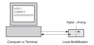
Figure C-1. Local analog loopback test.
